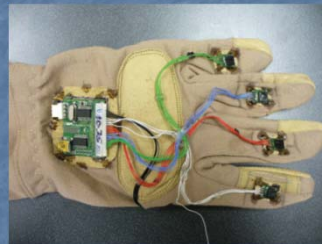
A data glove that uses accelerometers, gyroscopes, and magnetometers to capture information about each finger. (NuGlove Photograph courtesy of AnthroTronix)
