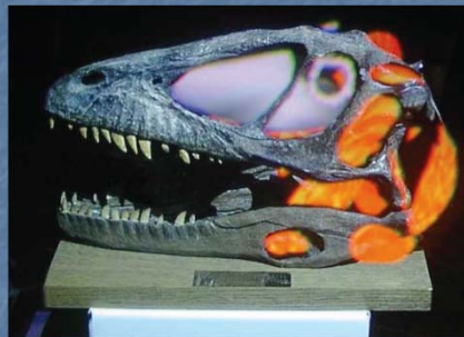
The Virtual Showcase, an augmented surface display that projects virtual information onto a physical 3D artifact, presenting a seamless integration of the physical object and virtual content. (Photograph courtesy of Oliver Bimber)
