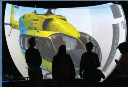
A curved, rear-projected surround-screen display that combines both hemispherical and cylindrical geometry. (Photograph courtesy of Digital Projection)
