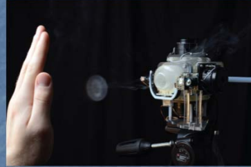
Vortex-based in-air tactile display. (Photograph courtesy of Ivan Poupyrev, copyright Disney, printed with permission)
