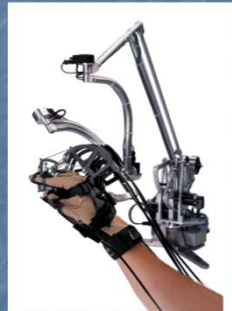
Combining ground-referenced and body-referenced force feedback (Photograph reproduced by permission of Immersion Corporation, © 2004 Immersion Corporation. All rights reserved)
