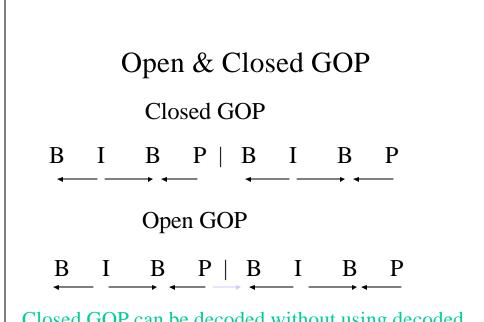
Closed GOP can be decoded without using decoded pictures from previous GOP.
