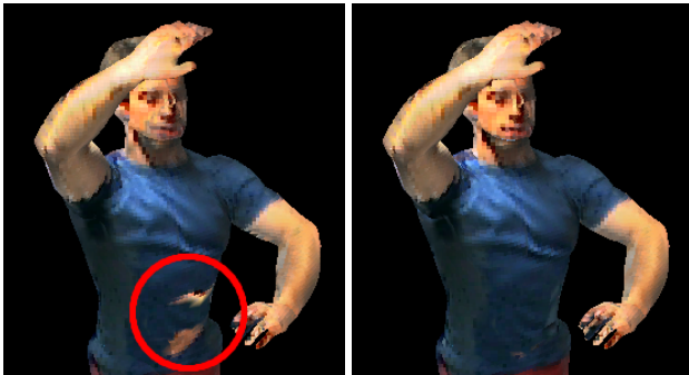
Figure 6: Incorrect texture projection (shown in red) is solved through a modified visibility calculation.
