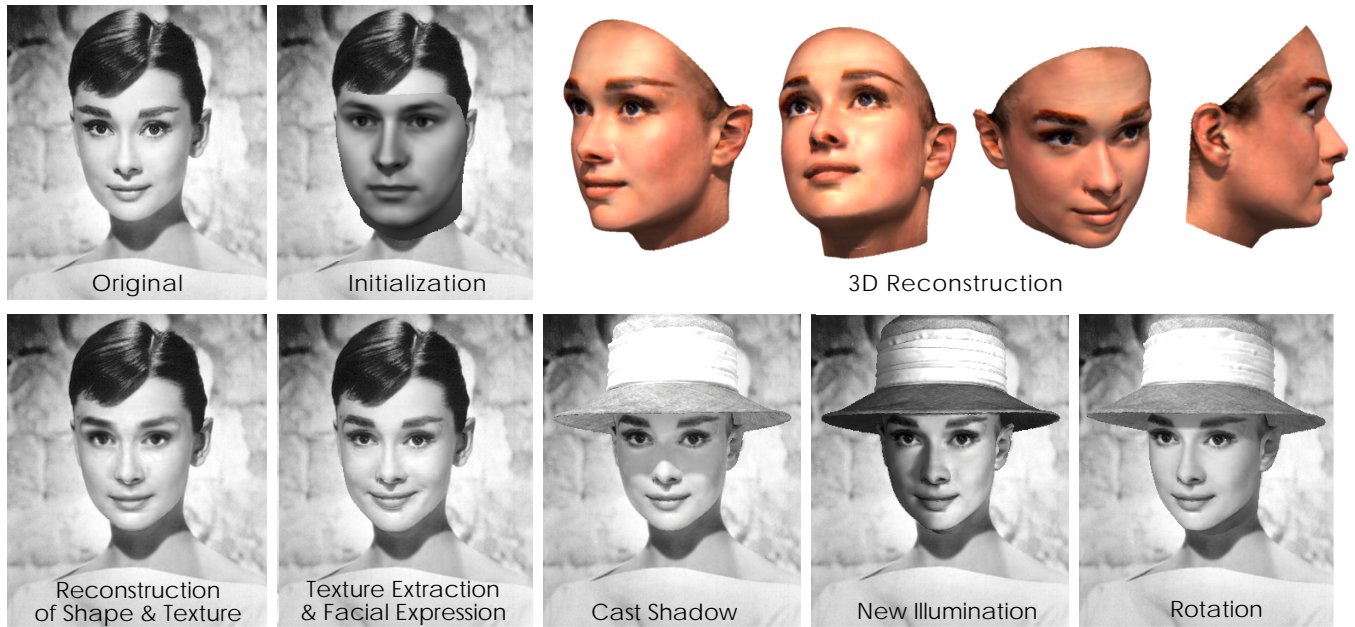
Figure 7: After manual initialization, the algorithm automatically matches a colored morphable model (color contrast set to zero) to the image. Rendering the inner part of the 3D face on top of the image, new shadows, facial expressions and poses can be generated.
