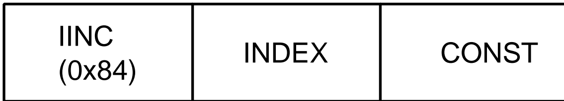
Figure 4-21. The IINC instruction has two different operand fields.
