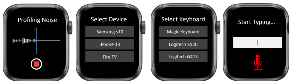
Fig. 2. An example GUI guiding through the application setup. First, the application performs noise profiling for the current typing session. Then, the user selects the device which the keyboard inputs will be forwarded. Next, the user selects the keyboard model. Once the application prepares the associated model, it starts listening for keystroke events.
