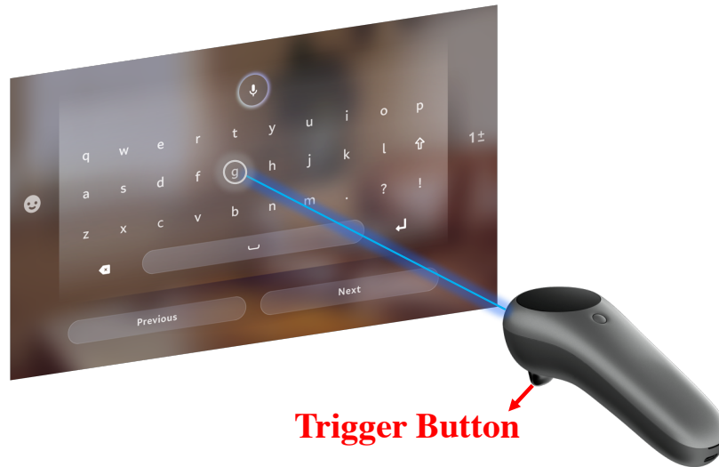
Figure 5.5: The system keyboard of Magic Leap 1, i.e., baseline keyboard. The targeting is done through moving the cursor via the ray coming out of the remote controller. The selection is done by pulling the trigger button at the back of the remote.
