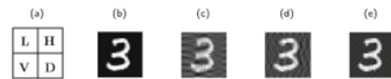
Figure 4. Local key-based sign flipping in the DCT sub-bands: a) sub-bands, b) original image, c) with a sign flipping in V, d) with a sign flipping in H, and e) image with a sign flipping in D.
