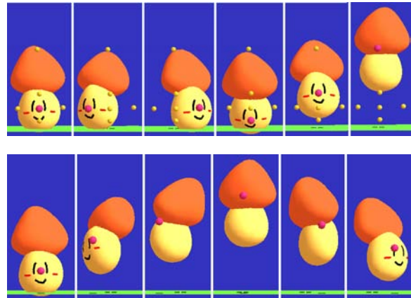
Figure 1: Spatial keyframing with six key poses (top) and an example animation sequence using it (bottom). The user associates each pose with a location in space (yellow markers) in a preparation phase. During performance, the user moves the control cursor (red sphere) and the system synthesizes an animation sequence by blending nearby poses.
