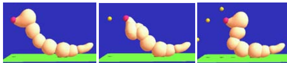
Figure 7: Initial pose (left), standard IK result (middle) and IK with spatial keyframing (right). Standard IK can produce very strange poses after continuous operation. In contrast, IK with spatial keyframing returns stable results regardless of previous pose.
