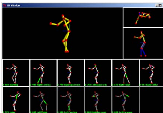
Figure 2 Our system provides a suggestive interface that allows the user to quickly guide reconstruction of the character's 3D pose. The currently estimated best pose is shown above and thumbnails of alternate poses are shown below. Clicking on a thumbnail flips the towards/away direction (with respect to the viewer) of a single bone in the 3D reconstruction.
