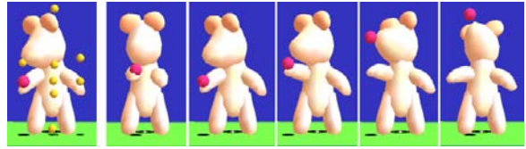
Figure 3: Juggling. The user first sets the nine key poses as shown on the left. As the user drags the control cursor, the character performs a smooth motion as shown on the right.
