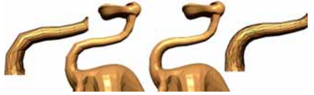
Figure 10: When performing significant deformations, the result can appear jagged if the input mesh is too coarse. Adaptive mesh refinement removes these artifacts.
