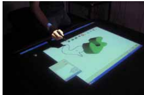
Figure 7: Our sketch-modeling interface is designed to support non-modal input devices, like this touch-sensitive horizontal tabletop display.
