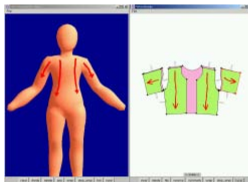
Figure 3: A screen snapshot of the system. Pink is the inside surface of the cloth, green is the outside, and the small gray lines indicate sewing constraints applied by the user.
