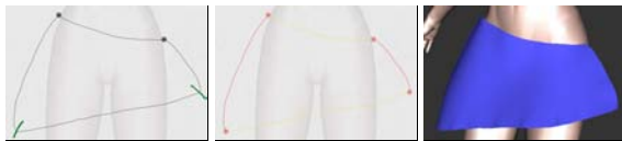
Figure 3: (left) The user drew the outline of the skirt without sharp corners at the bottom, and the corner-detector failed to put breakpoints there. The user therefore makes gestures (overdrawn in green here) to indicate the need for new breakpoints. (middle) The new breakpoints have been inserted. (right) The skirt is reconstructed.
