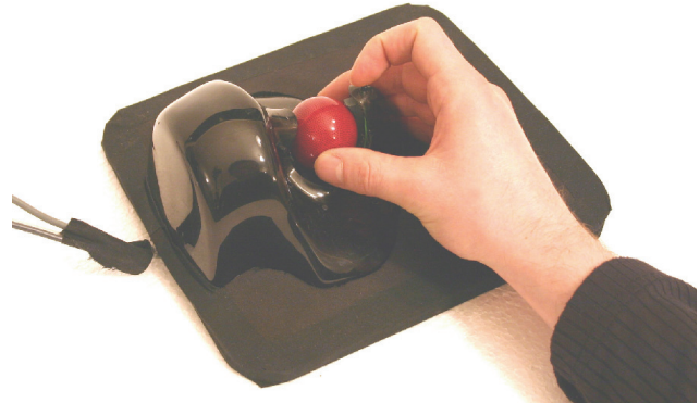
Figure 10: A GlobeFish prototype providing comfortable access to the 3-DOF rotations.
