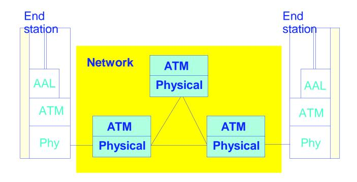
An ATM network provides an ATM layer connecttivity among ATM end stations
