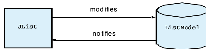
Fig. 3.11 JList and ListModel delegate-model architecture.
