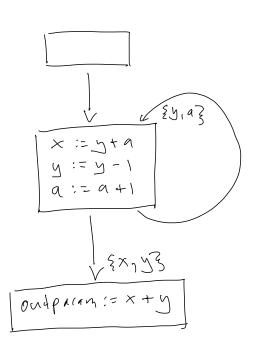
$$\text{IN}[B] = \bigcup_{P \text{ a predecessor of } B} \text{OUT}[P]$$
