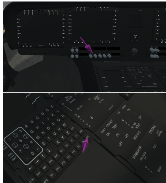
Figure 2: The interaction cues we employed in our user study. The 3D Arrow look cue (Top) directs users to where the target is located with respect to where they are looking. The 3D Arrow pick cue (bottom) distinguishes, out of the target candidates, which target is the one requiring attention.
